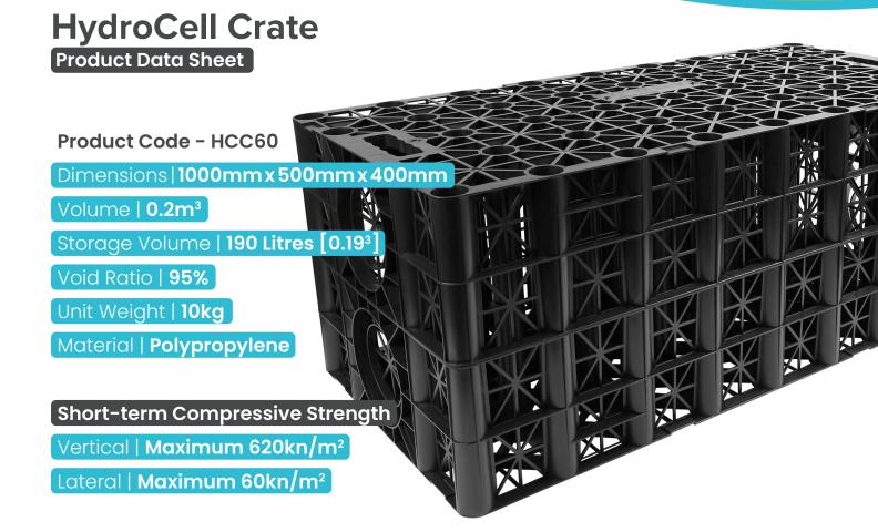
I HydroCell crate systems are used in stormwater retention, attenuation or infiltration applications. It also offers use in landscaped and deep soakaway applications.
